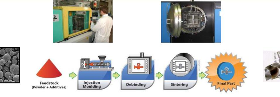
PIM technology allows to the production of high precision small parts without necessary to post-machining, with a significant cost reduction.
